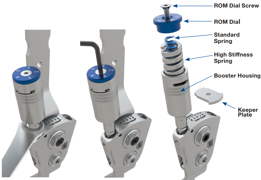
Figure 4. Adjust the booster to 15° ROM.
