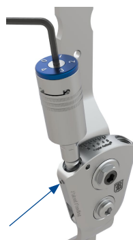
Figure 3. Loosen the ROM Dial screw using the 2mm adjustment wrench and zero the ROM setting by turning the blue ROM dial. The ROM lock set screw serves as a reference for this adjustment.
